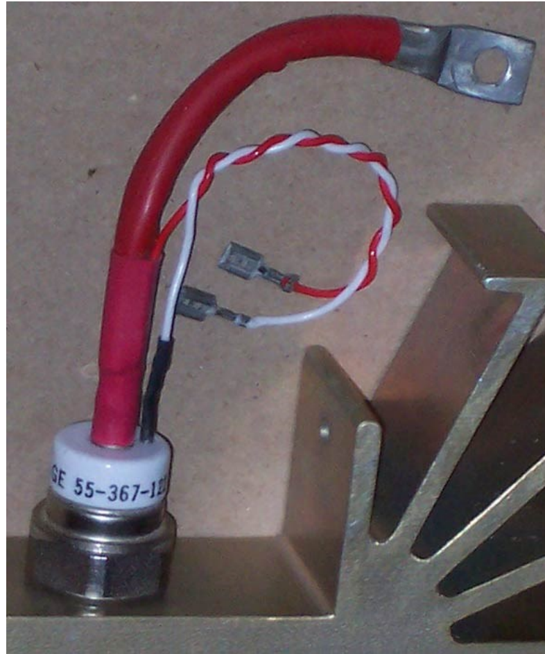
SCR, rated about 100 amperes, 1200 volts, 1/2 inch stud, photographed by C J Cowie. Uploaded on 4 April 2006.
